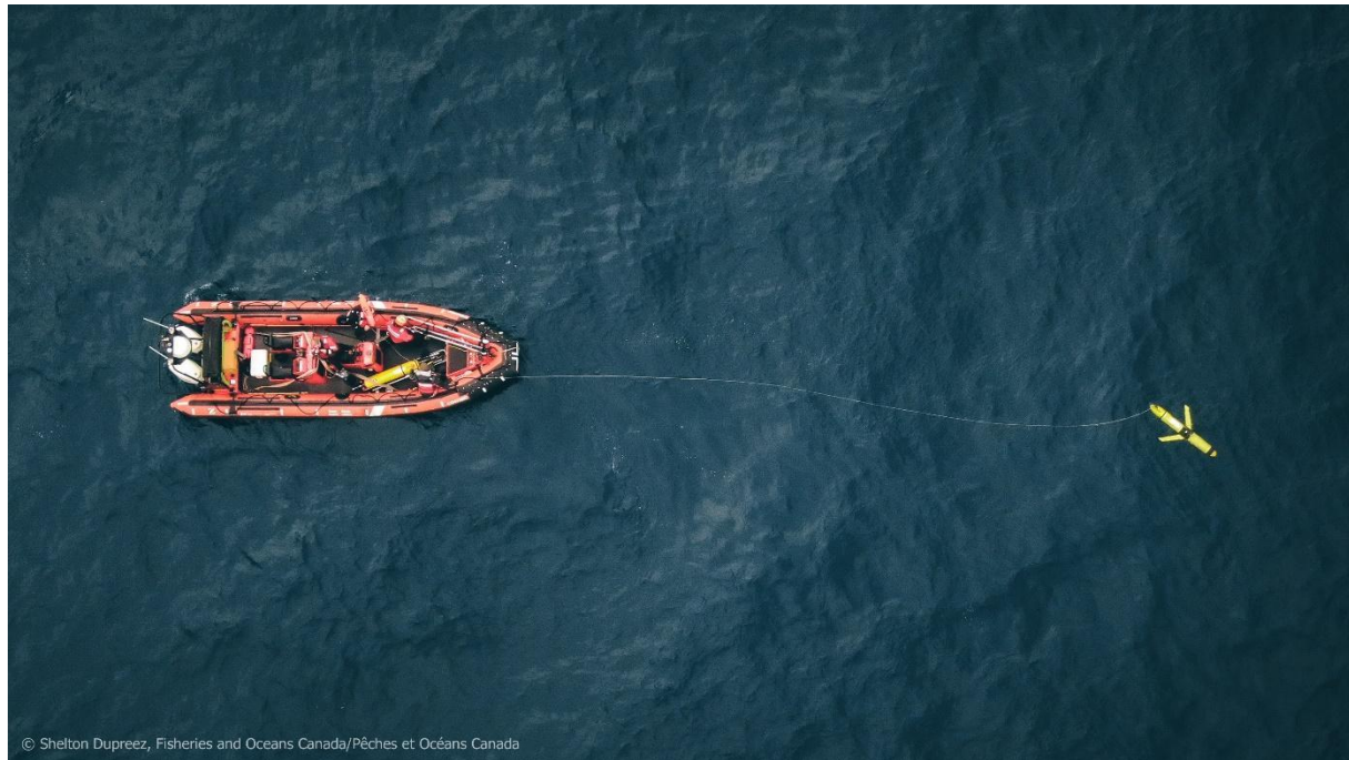
© Shelton Dupreez, Fisheries and Oceans Canada/Pêches et Océans Canada A glider deployed near Explorer Seamount by the Canadian-Pacific Robotic Ocean Observing Facility (C-PROOF) team.
